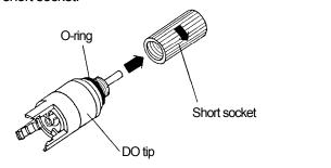
3 Attach DO tip to DO electrode body.
